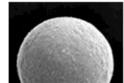
granulated zirconia averg. XRD-size 27 nm
