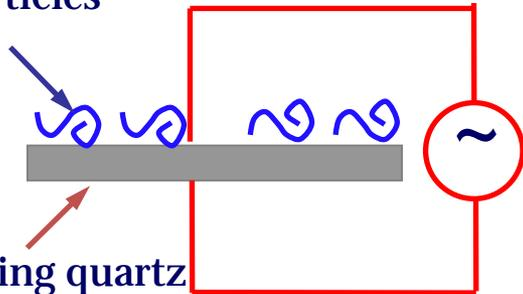
Oscillating quartz crystal detector
